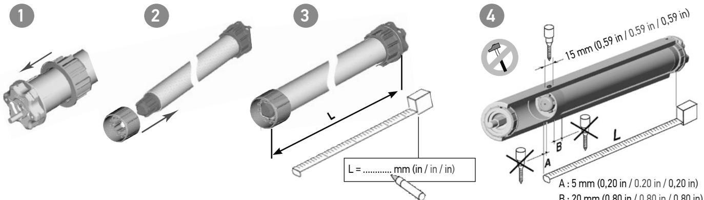
**3****FR** Installer le tube sur ses supports**EN** Install the tube on the brackets**IT** Montare il tubo sui propri supporti
